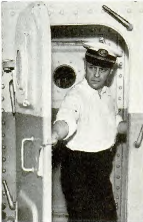
An emergency squad ready to battle disaster at sea Entering engine room through double-door air lock
